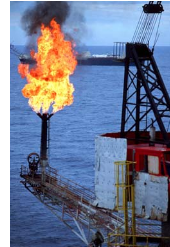
During crude oil production some wells burn off well gases as a safety precaution. Other rigs use the natural gas to power generators.
