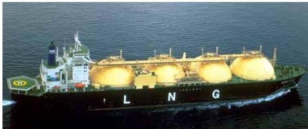
As a method of transport, natural gas is cooled and shipped in bulk as LNG.
